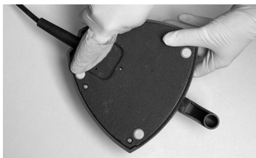
Figure 60 – Cleaning of foot control “rubber feet”
