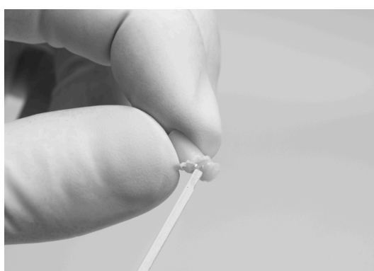
Figure 63 – Non-polymerized material is removed from composite test plug
