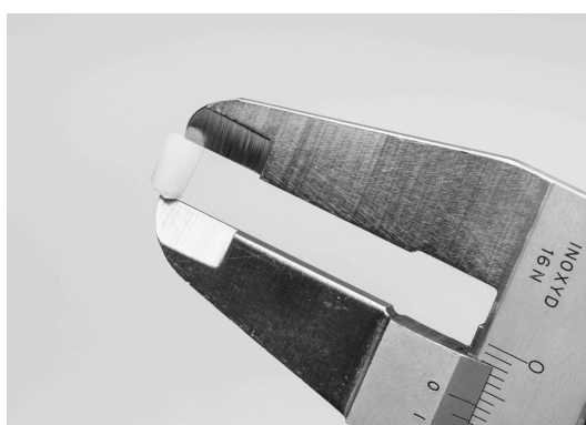
Figure 64 – Measuring the depth of the test plug
