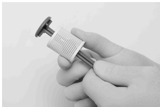
Figure 55 – Removing filter cartridge from filter holder
