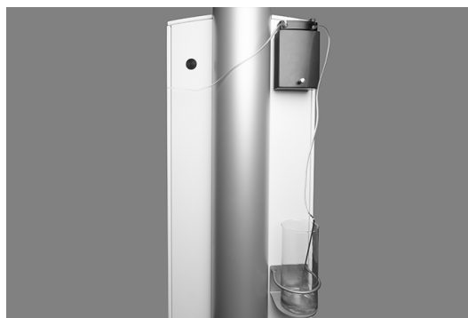
Figure 24 – Placing the reservoir
